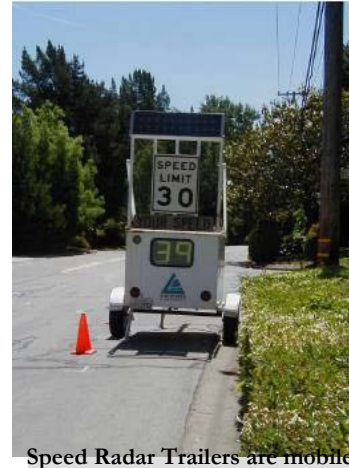
Speed Radar Trailers are mobile devices for encouraging and enforcing slower vehicle speeds
