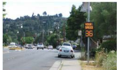
Variable Speed Feedback Signs show vehicle speeds in real-time as they pass the sign
