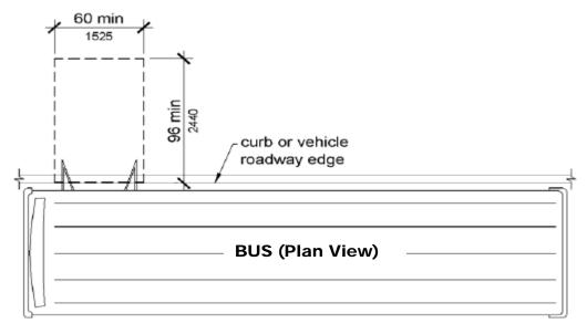
Figure 810.2.2 Dimensions of Bus Boarding and Alighting Areas
