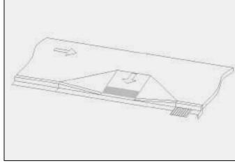
**Figure 5: Perpendicular Curb Ramp**
