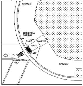
**Figure 4: Curb Ramp Components**
