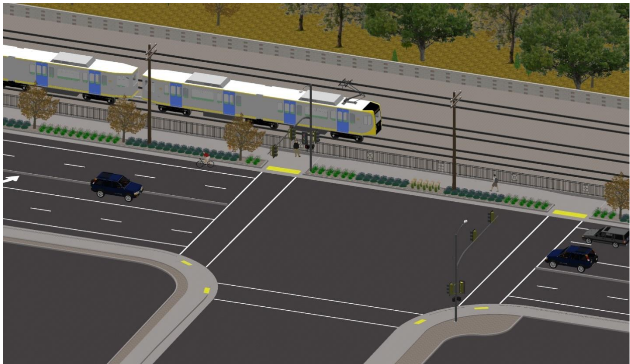
Rendering of improved pedestrian crossing and possible safety railing installed between the sidewalk and light rail tracks.
